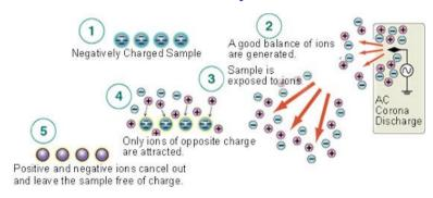
If the ionizer supplies a poor balance between positive and negative ions, it could prevent achieving a neutral charge or cause a reverse charge.
